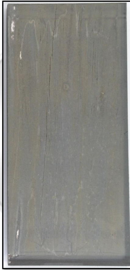
Figure 2. Specimen 1 – After exposure to 6,109 hours of Xenon-arc Simulated Weathering Test
