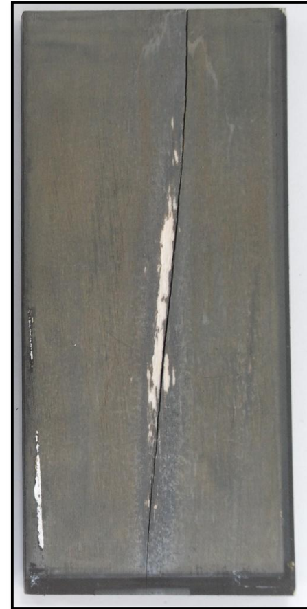
Figure 3. Specimen 2 – After exposure to 6,109 hours of Xenon-arc Simulated Weathering Test
